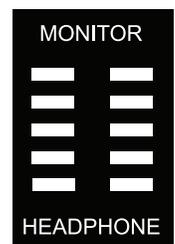
When in Monitor mode, press the MONITOR button to change the selected output. Press again to switch to the other output.
